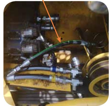
Split factory quick couplers, remove quick coupler end (screw style is the return YELLOW, push style is the pressure BLUE) install the short pipes as shown, install T fittings, re install factory lines to the through side of the T and then install the lines with the elbows to the legs of the T fittings as show.
