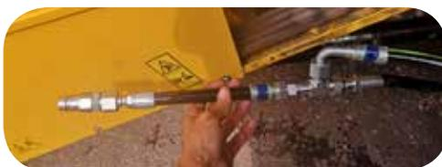
Connect the pressure and return lines that run under the cab to the ones running to the valve.
